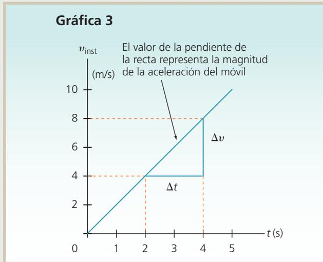
$$a = \frac{\Delta v}{\Delta t} = \frac{8 \frac{\text{m}}{\text{s}} - 4 \frac{\text{m}}{\text{s}}}{4 \text{ s} - 2 \text{ s}} = \frac{4 \frac{\text{m}}{\text{s}}}{2 \text{ s}} = 2 \frac{\text{m}}{\text{s}^2}$$
