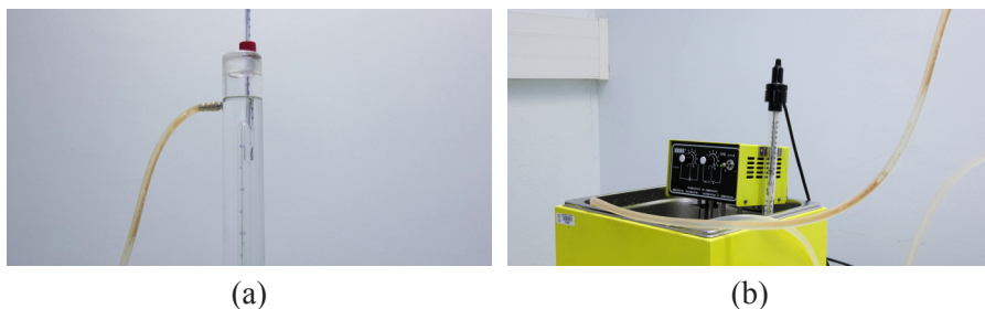
Figure 5. (a) Water concentric tube surrounding the measuring tube; (b) Thermostatic bath.
