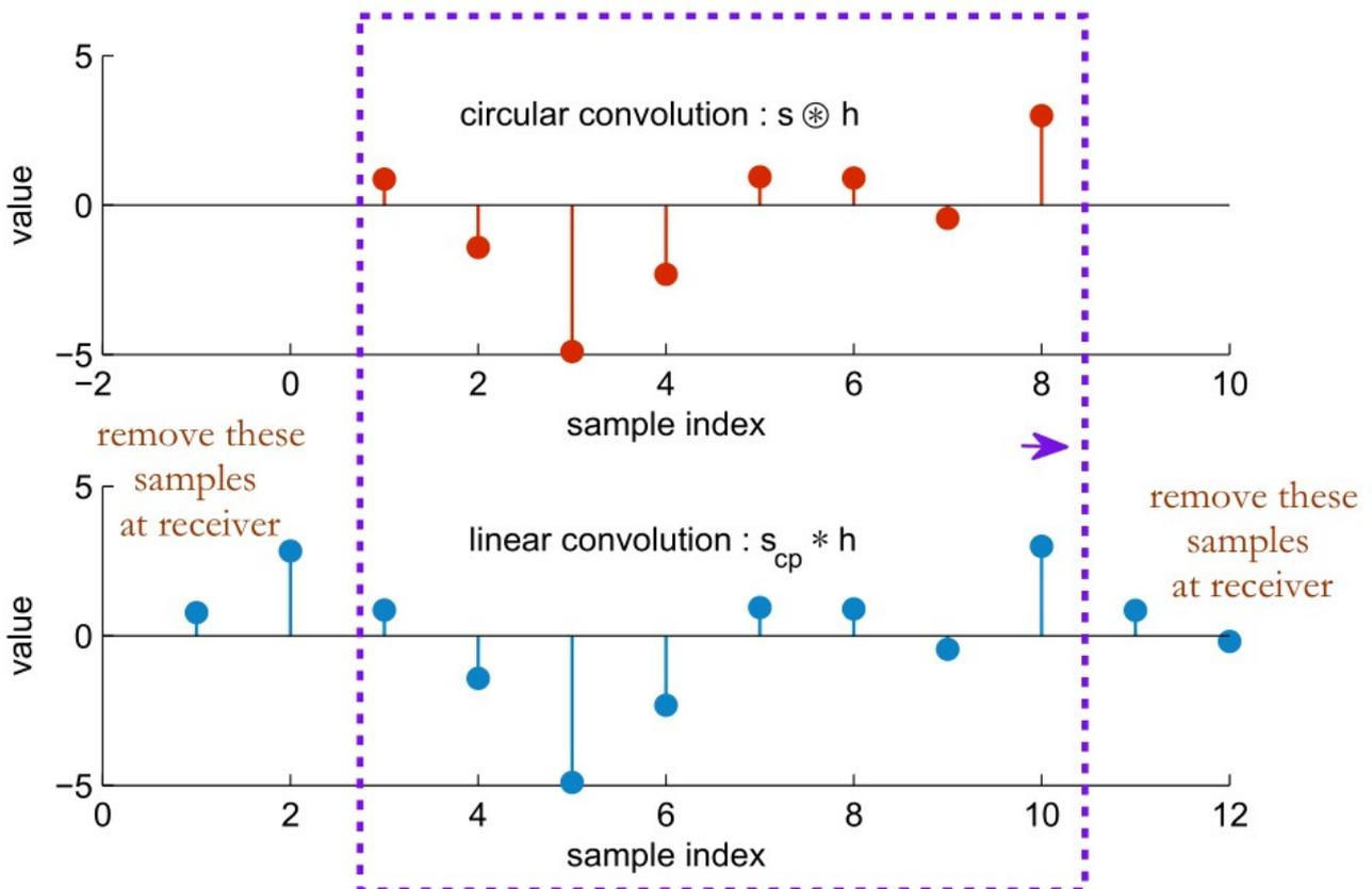
We have just tricked the channel to perform circular convolution by adding a cyclic extension to the OFDM symbol.
