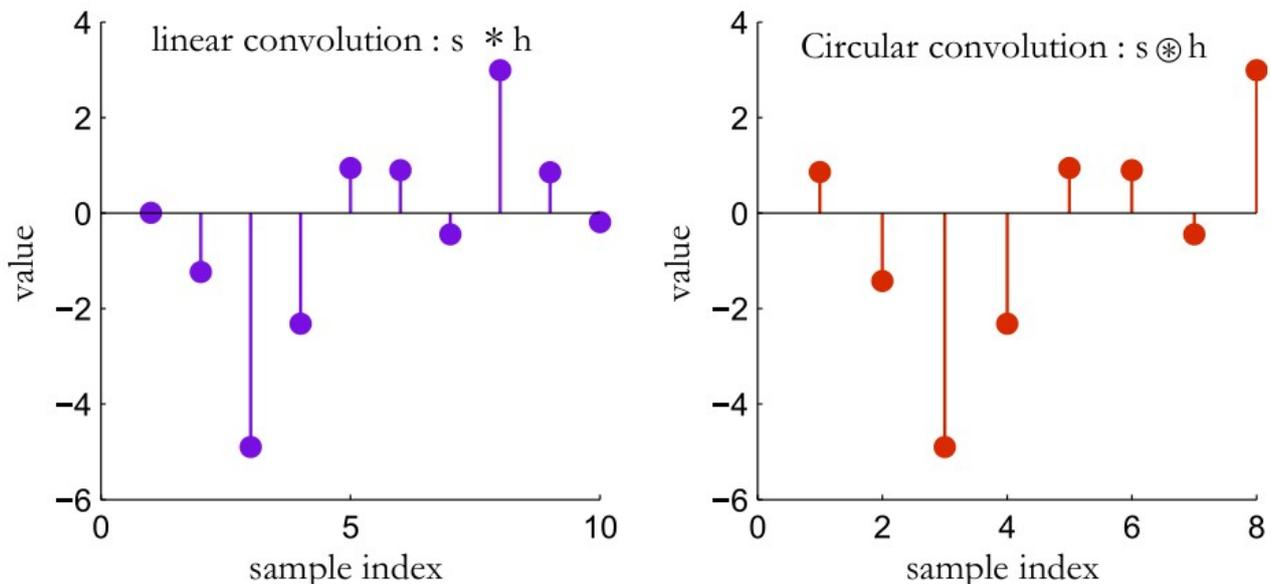
We note that the linear convolution and the circular convolution do not yield identical results.
