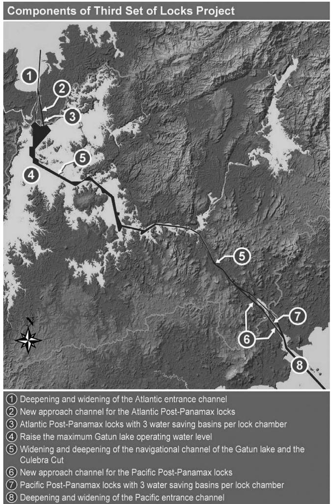
**Fig. 2.** Panama Canal Expansion Program [Reprinted with permission from Autoridad del Canal de Panamá (ACP) 2006]
