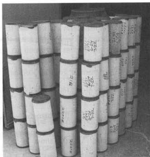
Standard capped cylinders ready for testing.
