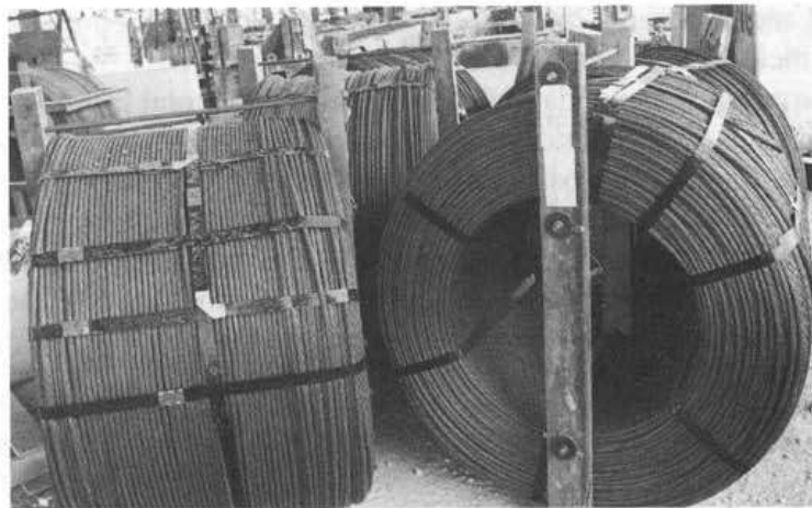
Seven-wires prestressing strands (shipped in coils as shown).
