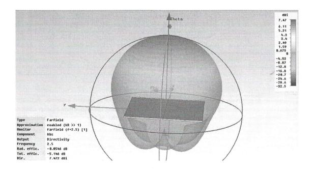
You can see that the maximum power is radiated in the positive z-direction. Note that there are several other options available to plot a farfield: the Polar plot, the Cartesian plot and the 2D plot.
