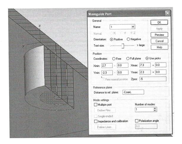
Here, you have to choose how many modes should be considered by the port. For a simple coax port with only one inner conductor, usually only the fundamental TEM mode is of interest. Thus, you should simply keep the default setting of one mode.
