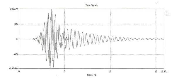
This plot shows the incident and reflected wave amplitudes at the waveguide port versus time. The incident wave amplitude is called i1 (referring to the port name: 1) and the reflected wave amplitude is o1,1. As evident from the above time-signal plot, the patch antenna has a strong resonance that leads to a slowly decreasing output signal.
