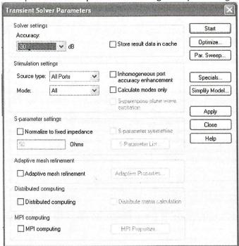
We recommend using reasonably large bandwidths of 20% to 100% for the transient simulation. In this example, the S-parameters are to be calculated for a frequency range between 2 and 3 GHz. With a center frequency of 2.5 GHz, the bandwidth (3 GHz - 2 GHz = 1 GHz) is 40% of the center frequency, which is inside the recommended interval. Thus, you can simply choose the frequency range as desired between 2 and 3 GHz.
