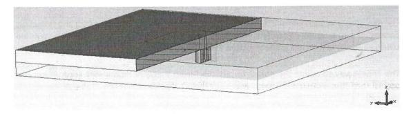
To finish the 3D model, the last thing to do consists on removing the part of the ground plane that is shortcircuiting the coaxial feed. Select the ground plane and click *Objects in Boolan Insert* (inner conductor). Then select the 3 elements of the coaxial feed (inner conductor, dielectric and outer conductor) and press enter. Now the ground plane has a circular hole to prevent blocking the RF signal travelling from the coaxial and the patch antenna model is complete.
