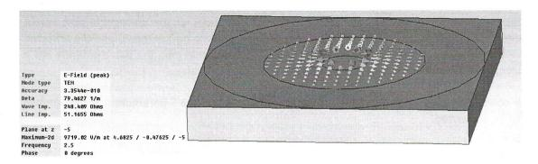
In this case, as expected, the field corresponds to the dominant mode in a coaxial waveguide. The plot also shows some important properties of the mode such as mode type, propagation constant and line impedance. Here, you can see that the port impedance is approximately 50 Ohms, which is agrees with the specifications of the SMA connector.
