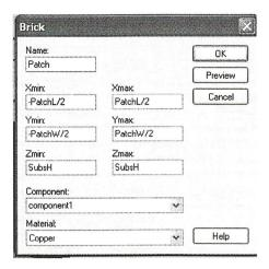
The basic structure of the patch antenna is already created. You can now modify the value of any parameter (*PatchL*, for instance), click *F7* and the model will be automatically updated.
