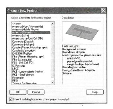
This template automatically sets the units to mm and GHz, defines the background material to vacuum and selects appropriate boundary conditions (see chapter Boundary Conditions). Because the background material has been set to vacuum, the structure can be modeled just as it appears on your desk.
