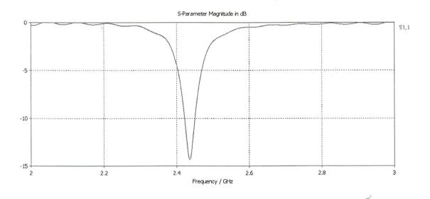
It is possible to precisely determine the operational frequency for the patch antenna. Activate the axis marker by pressing the right mouse button and selecting the *Show Axis Marker* option from the context menu. Now you can move the marker to the S11 minimum and pinpoint a resonance frequency for the patch antenna of about 2.45 GHz.
