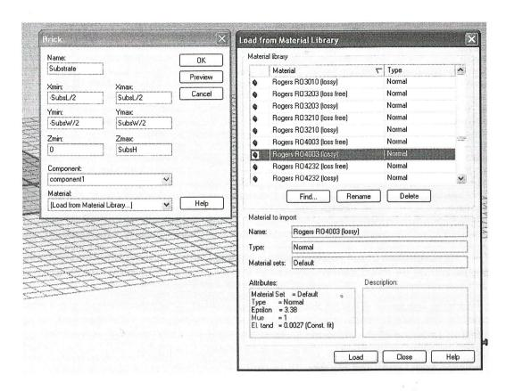
We specify the name of the brick: 'Substrate'. The coordinates of the brick can be specified using either numerical dimensions or parameters. In this case, we will use the previously defined parameters. The material can be directly selected from a *Material Library*. We will use a standard substrate *Rogers RO4003(lossy)*.
