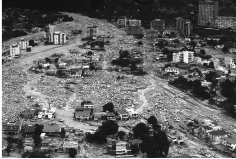
Fig. 1.1. Example of the consequences of a slope instability. Aerial view of debris-flow deposition resulting in widespread destruction on the Caraballeda fan of the Quebrada San Julián. Avulsion of the main channel (left side of photo) resulted in deposits up to 6-m in thickness and totaling about 1.8 million cubic meters of bouldery debris. Secondary new flood channels are visible through center of fan to the lower right of photo.
