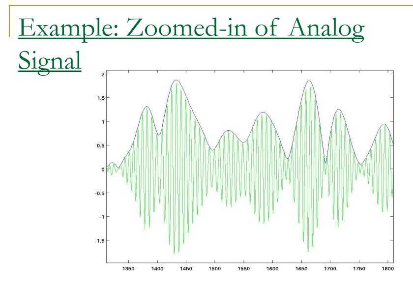
Analog signal modulated onto a carrier
